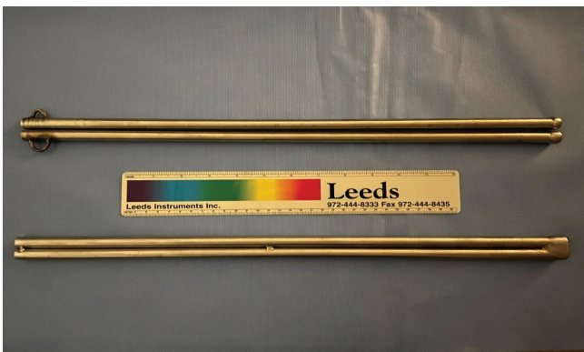
Figure 2. "Cervitomes" used for amputation of the mare's cervix. The instrument above the ruler is a pair of stainless-steel tubes that were taped together for the first application of this procedure. The instrument below the ruler used for subsequent procedures was fabricated with a hardened head to mimic the Utrecht model fetotome.
