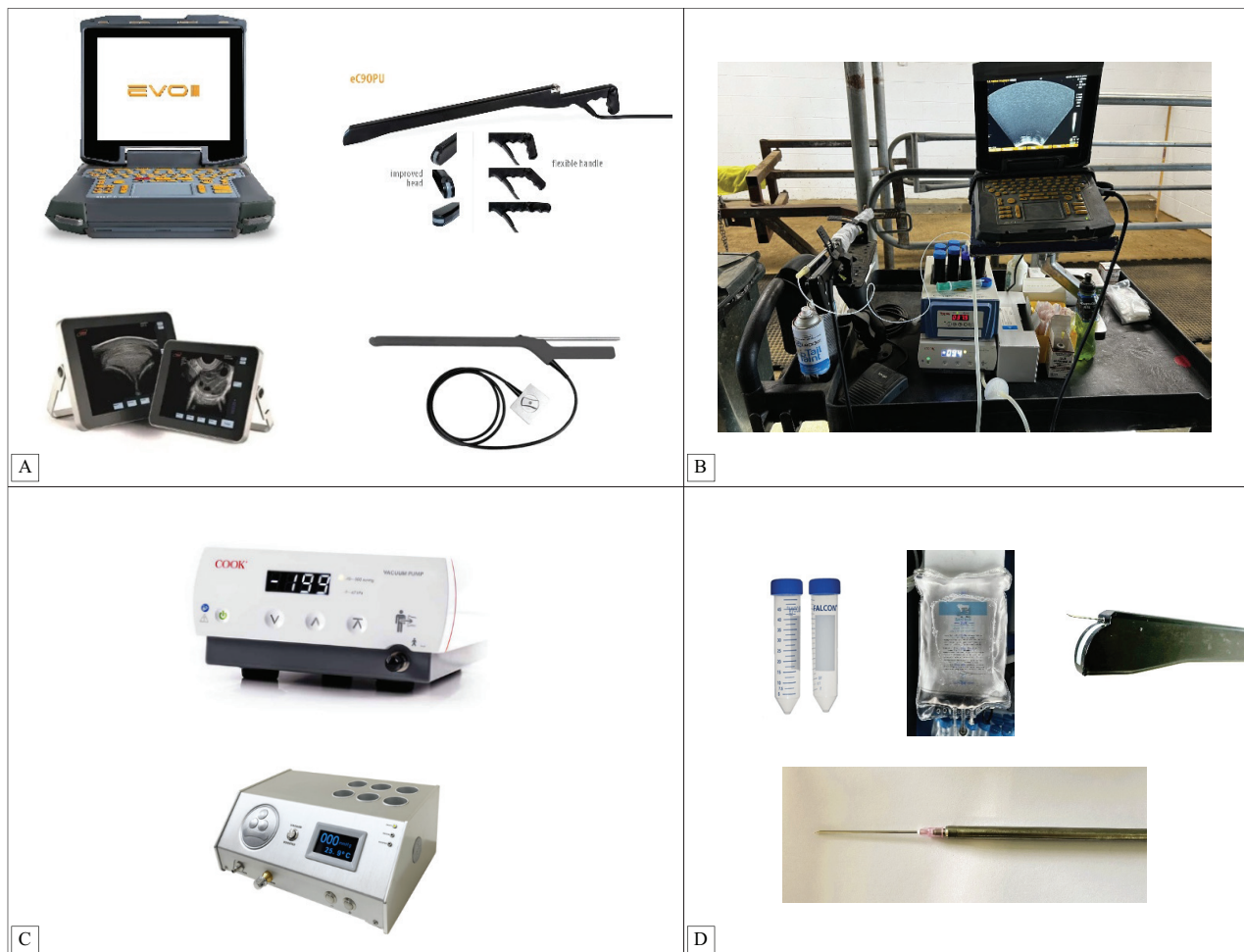
Figure 4. Equipment necessary to perform OPU in donor cattle. A. Examples of 2 modern ultrasonographic machines/units (on left) capable of attaching to a transvaginal probe (on right)) for imaging ovaries; B. First author's complete setup; C. Example of digital vacuum pumps (Cook medical [above], WTA technologies [below]) able to control and select variable vacuum pressures and flow rates; and D. Necessary accessories (e.g. aspiration collection centrifuge tubes [Falcon] commercial flush media [Boviflush, Minitube] supplemented with 5 IU/l heparin, metal needle rod with detachable long-bevel needle (in this case, 3 inch 18 gauge, [SUPRA Minitube Australia])
